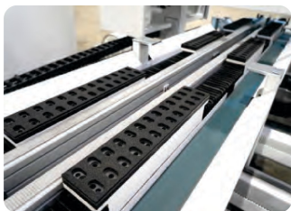
Vacuum sucker working table Adjust sawing according to panel size, prevent destroying the working table
