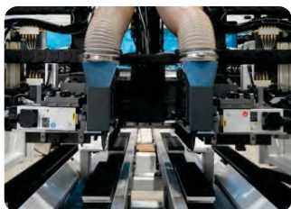
Longitudinal Saw Unit Servo-driven, scoring saw adjust based on panel thickness to ensure the precision sawing
