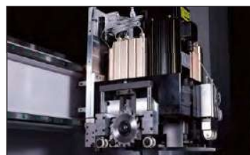
Saw Blade hogging 55-880mm straight groove
