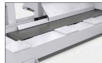
Belt conveyor dust collection Centralized remove all dust which fall into machine.
