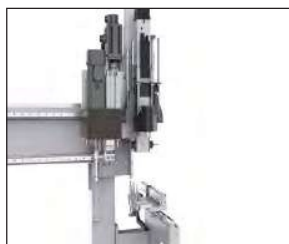
5 type ATC, Various Tool available, Use for hogging, Milling, Lamello Connector Working
