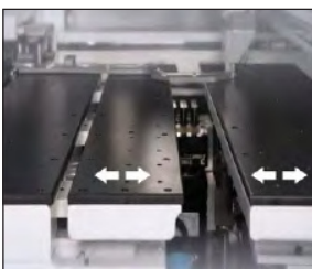
Double Translation air Floating table: Can move flexibly according to the hole position to improve the drilling accuracy
