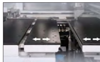
Double translational air flotation table (patent)
