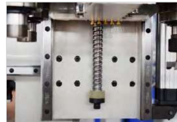
Transmission mechanism Transmission mechanism: z-axis adopts ball screw. with high movement precision and compact structure.
